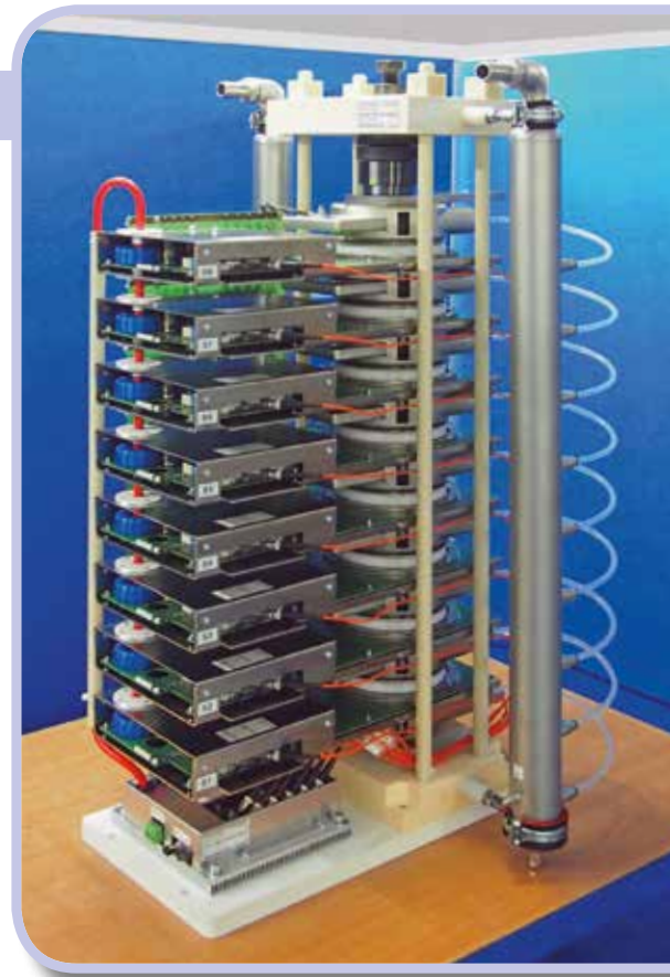
Example of a 20kV, 13kA 300Hz, 10kA/ \mu s Switch Assembly
